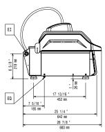
Electrical inlet (power) EO Electrical Outlet
